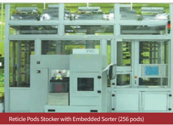
Reticle Pods Stocker with Embedded Sorter (256 pods)
